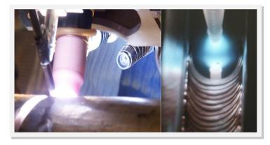
Redman Controls MC500 and MC500S video camera unit is designed to image weld arcs and provide the user with the perfect tool for weld arc monitoring inspection especially from remote or inaccessible places.
